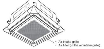
The indoor unit's intake grille can be removed for easy cleaning and maintenance
