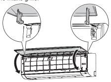
3. Press 4 places on the intake grille to close it completely.
