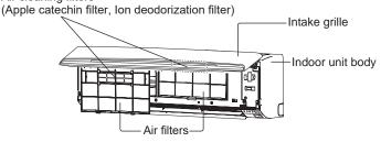
The frequency of the cleaning is as shown in the following table.
