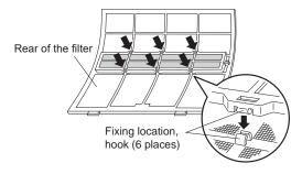
**11.** Replace the air filters and close the intake grille. Refer to steps 4 ~ 5 of "Cleaning air filter".
