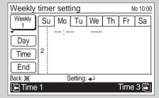
Press the [Enter button]. Then select [Weekly 1] or [Weekly 2] with the [Cursor button (Up/Down)], and press the [Enter button].
