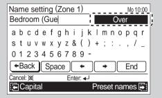
4 Set the cursor to [End] with the [Cursor button], and press the [Enter button] to finalize the name registration.
