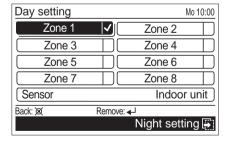
Select zone to be registered in the group with the [Cursor button]. When you press the [Enter button], a check mark is displayed.
