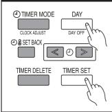
Press the DAY (DAY OFF) button and TIMER SET button simultaneously for 2 seconds or more to activate the child lock function and lock all of the buttons on the remote controller except the START/STOP button, SET TEMP. buttons, MODE button, and FAN button. Press the buttons again for 2 seconds or more to deactivate the child lock function.
