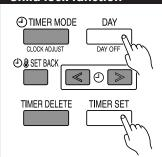
Press the DAY (DAY OFF) button and SET button simultaneously for 2 seconds or more to activate the child lock function and lock all buttons on the remote controller. Press the buttons again for 2 seconds or more to deactivate the child lock function.
